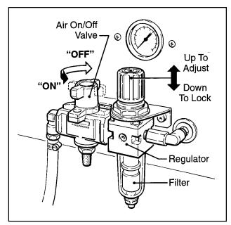
Figure 3-3 - "On/Off" Valve/Regulator/Filter
